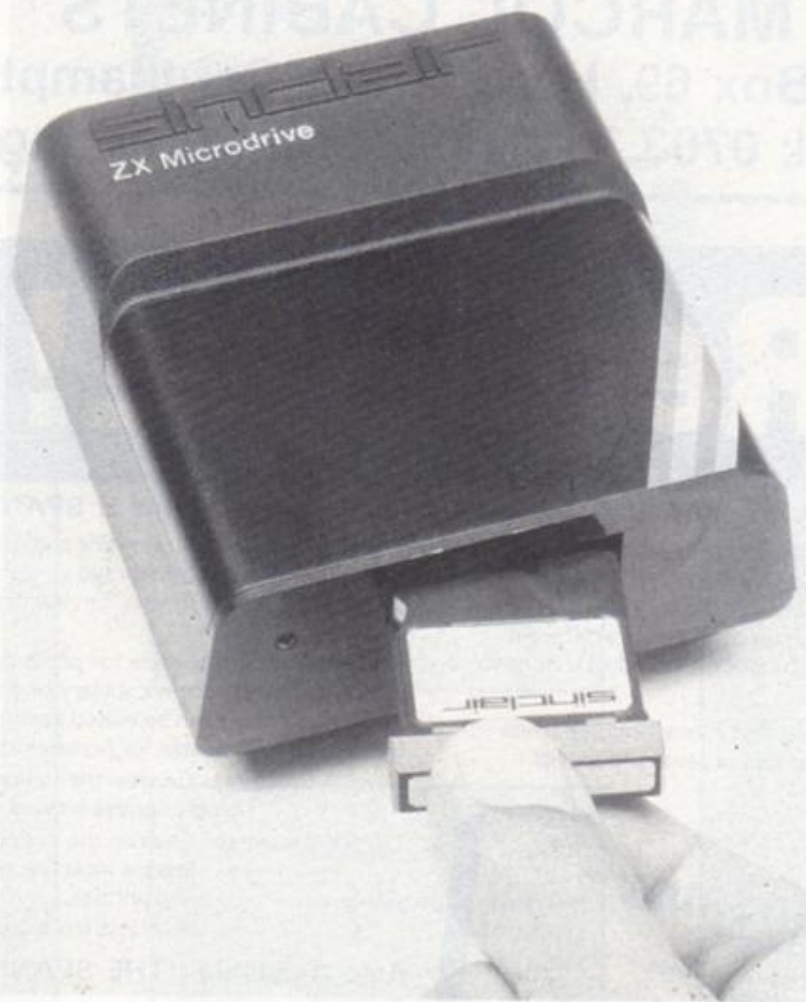
A tiny tape cartridge slots into Sinclair's Microdrive — make them work harder for you
